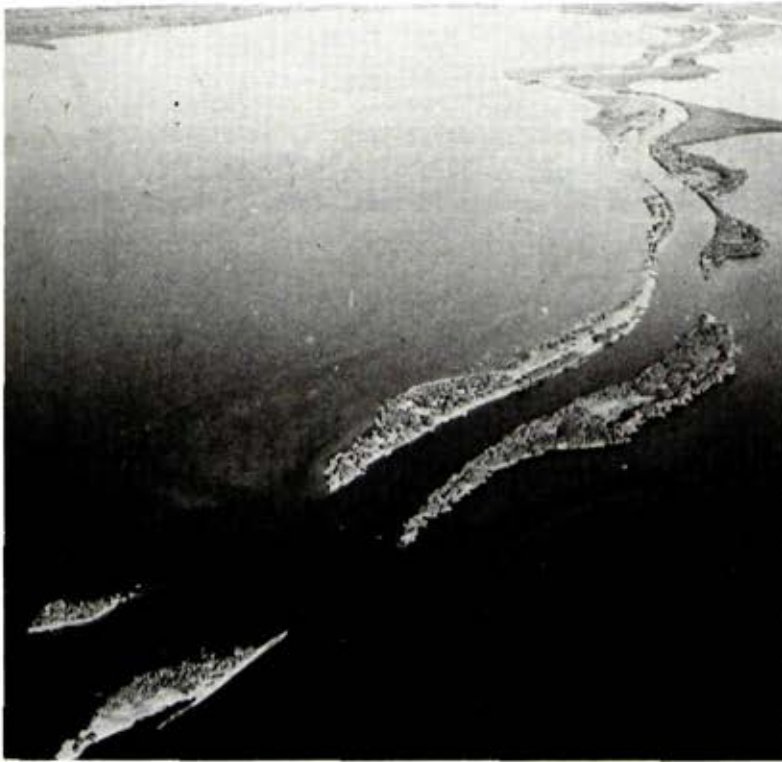
Parts of the Mitchell River silt jetties are submerged when Lake King water levels are high
