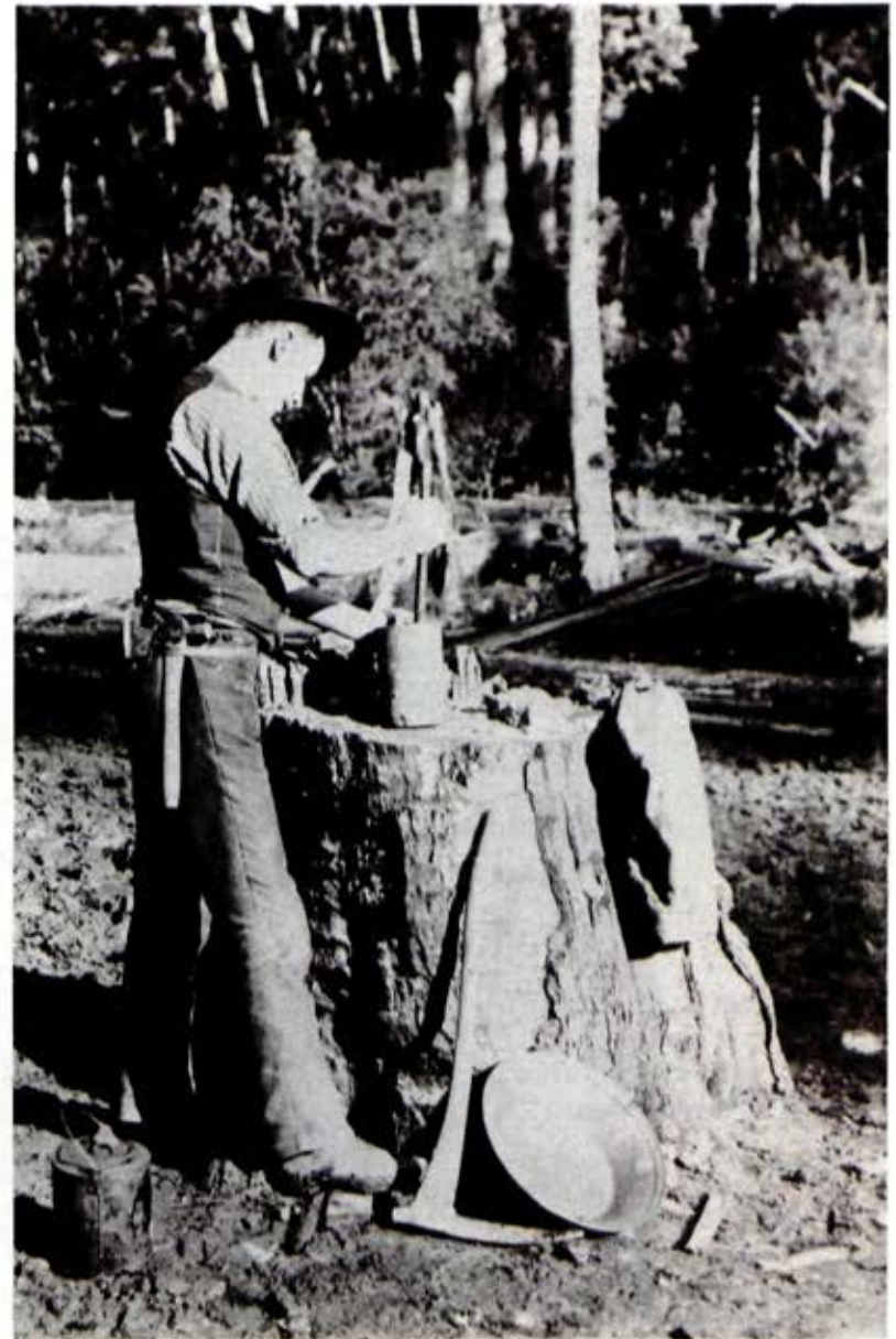
Miner crushing quartz in dolly pot
